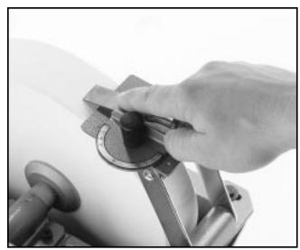
Figure 5. Proper sharpening position.
